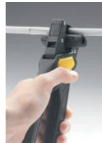
Round cut left and right of the longitudinal cut via 1/4 rotation of the stripper
